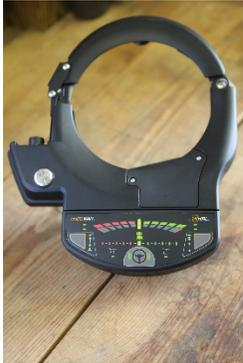
Wheelman™ Flex makes autosteering simple and affordable for every farm. The GPS controlled Wheelman Flex is dust and water proof (IP67 rated) and can easily be moved and used between other equipment, further reducing the cost of outfitting a farming operation with autosteering. The included guidance dashboard allows farmers to quickly define a repeatable field path and engage the Wheelman system to begin autosteering.
